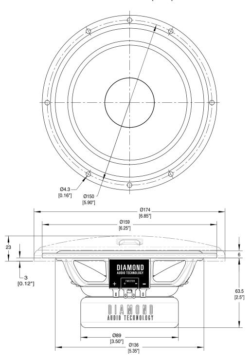
**M371i** General dimensions in millimeters and [inches]. Not to scale.
